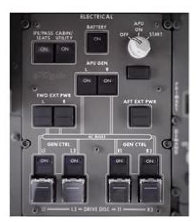
The engines are started using two electric starter units (not the bleed system!) and once the engine is running those same two starter units on each engine run as generators that power the four AC buses.
