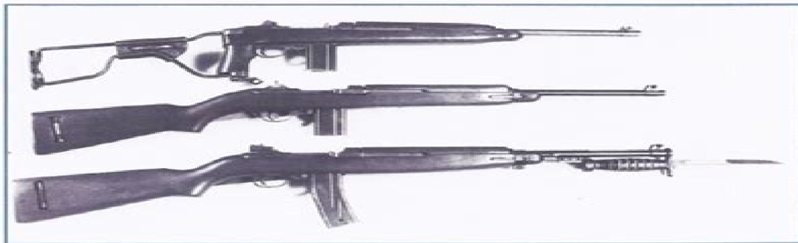
(Top to bottom) M1A1 carbine with stock in extended position; M1 carbine with all "early" features and 15-round magazine; M1 carbine with later (M12 type) parts, 30 round magazine and M1 bayonet.
