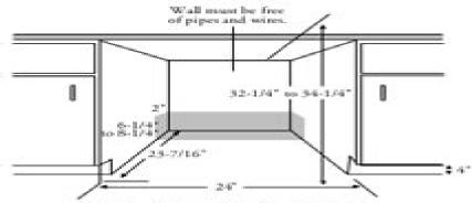
Electrical and water supply should oncer through the shaded area and come up through the right side of the machine. Maximum of 4" from the back wall and 8" from the floor.
