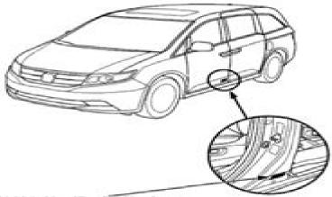
Vehicle Identification Number, Federal Motor Vehicle Safety Standard Certification, and Paint Code Label.
