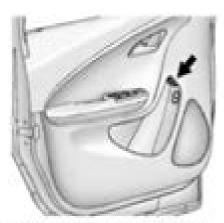
1. Press the fuel door button on the driver door for one second. A WAIT TO REFUEL message displays on the Driver Information Center.
