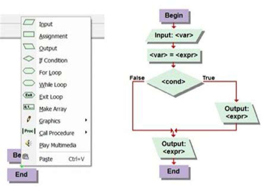
Fig. 1: Visual Logic tool showing how it guides the user to construct a runnable program.
