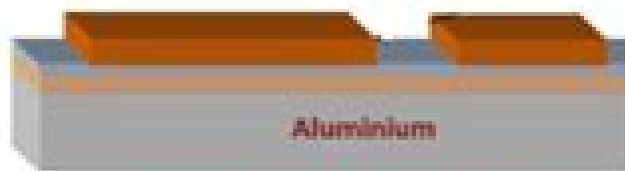
Aluminium Backed PCB
