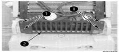
Remove the bolts (1) and pump guard (2) from the machine.
