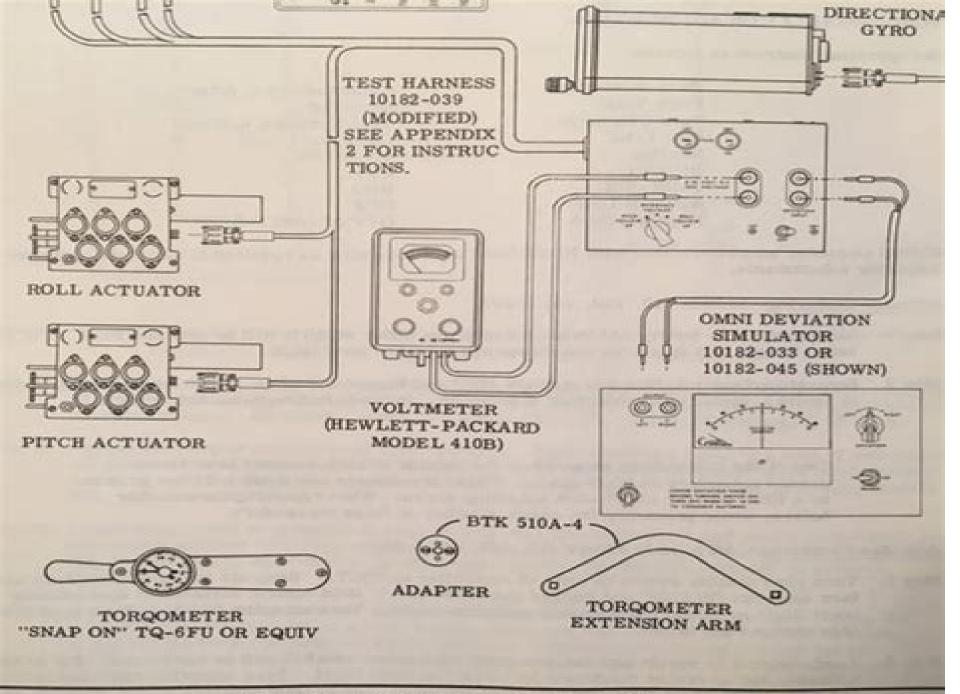
Figure 3-6. Bench Test Interconnection Diagram
