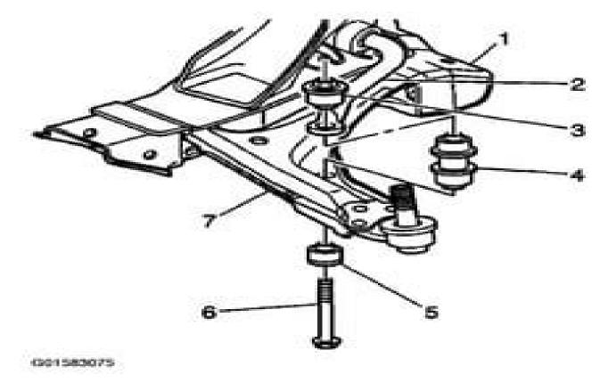
Fig. 4: Stabilizer Shaft Insulator Brackets Courtesy of GENERAL MOTORS CORP.
