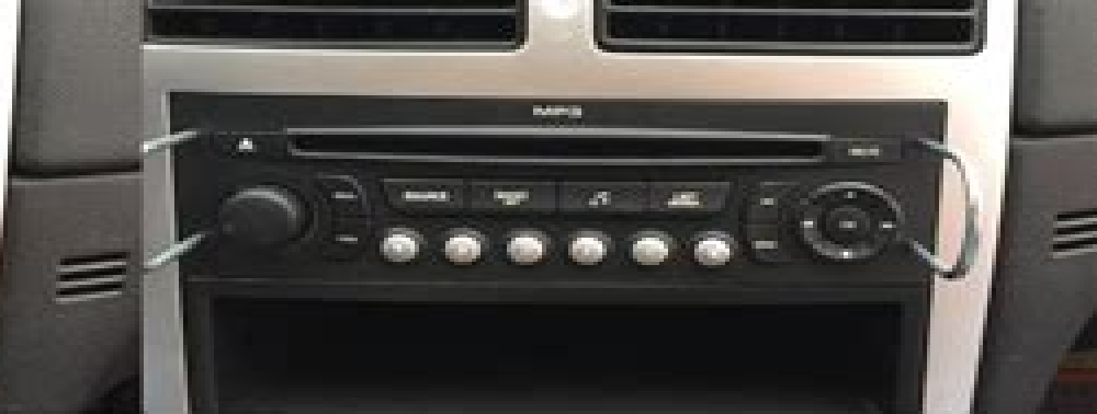
2. USING A U-SHAPED TOOL INSERT IT INTO THE MAIN UNIT REMOVAL HOLE
