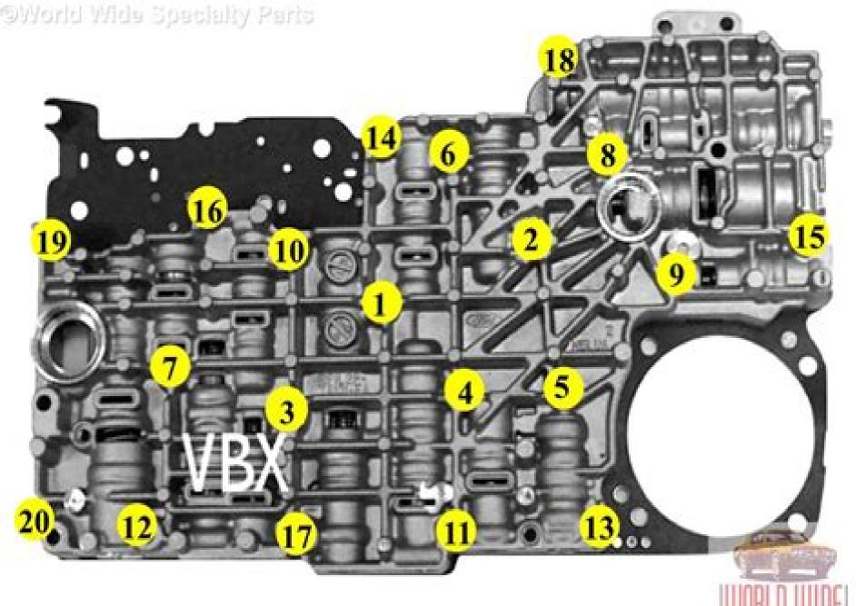
Torque Valve Body Bolts in Sequence Shown To 89 Inch
