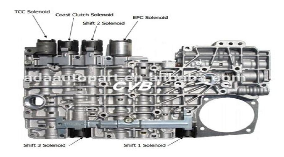
CVB# FD-3320 - 4R44E - 95-Up, 6 Solenoids CVB# FD-3321 - 4R55E - 95-96, 6 Solenoids CVB# FD-3322 - 5R55E - 97-Up, 6 Solenoids
