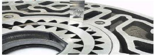
Outer gear to top-of-pocket clearance:
