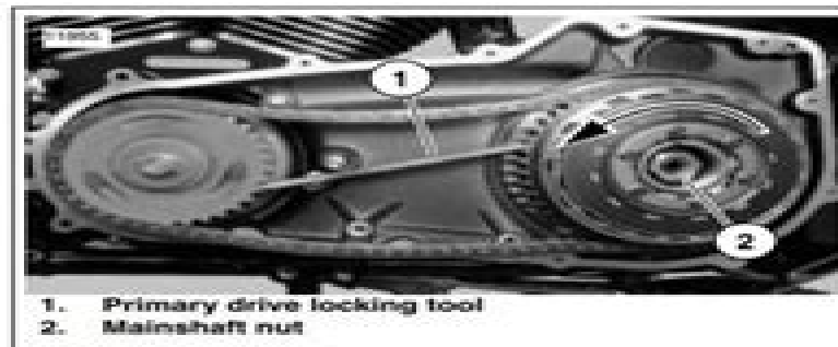
Figure 6-18. Installing Clutch Hub Mainshaft Nut
