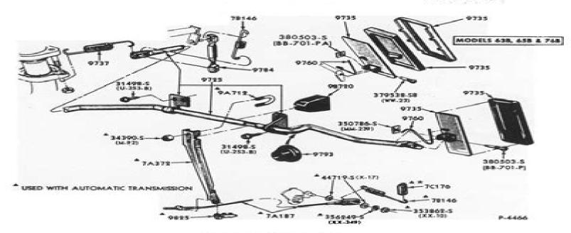
ACCELERATOR LINKAGE 1965/68 MUSTANG (6 CYLINDER 170, 200 ENGINES)
