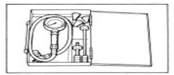
This compression gauge is used to measure the engine compression pressure.
