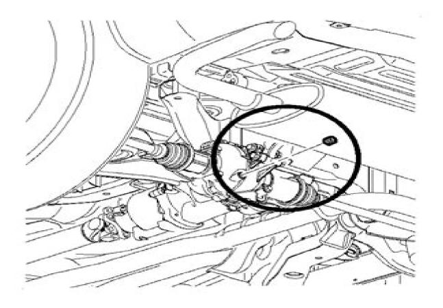
Fig. 3: Removing/Installing Fluid Fill Plug Courtesy of GENERAL MOTORS CORP.
