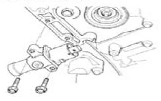
Align the holes on the rod and the housing of the auto-tensioner.
