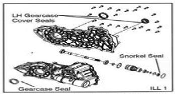
Reverse the disassembly procedure for the assembly of the snorkel shaft assembly.  Inspect the output gear assembly (A), replace bearings if needed. Inspect the 91T gear for nics, chips, or abnormal worn teeth.
