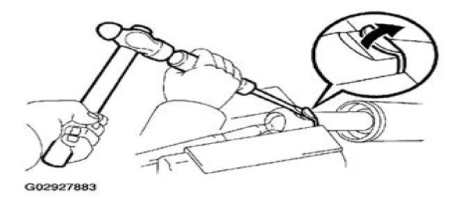
Fig. 9: Unstaking Claw Washer Courtesy of TOYOTA MOTOR SALES, U.S.A., INC.
