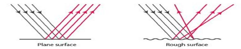
When a ray or beam of light falls on a smooth and polished surface an irregular reflection is observed when the light falls on a rough surface. As the surface is uneven, light rays from several points gets reflected in different directions, producing irregular reflections.
