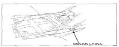
The color label is attached on the right side of the frame under the seat. When ordering color-coded parts, always specify the designated color code.
