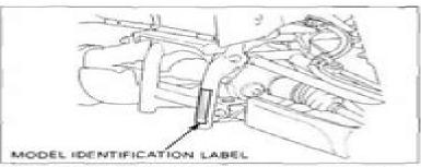
The model identification label is located on the left side frame down tube.
