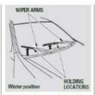
Adjust the wiper arms to the winter position by holding both arms as shown in the illustration at the same time. Pull on the arm, parallel to the windshield, until it locks in the higher position.
