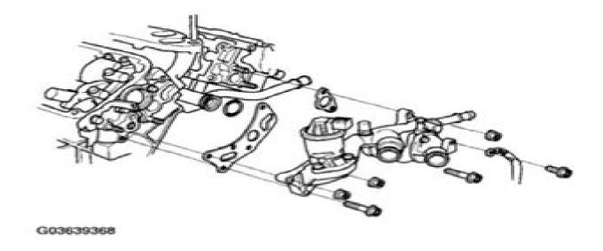
Fig. 90: Removing Water Passage Courtesy of AMERICAN HONDA MOTOR CO., INC.
