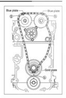
Install timing chain guide (2), then tighten bolts securely.
