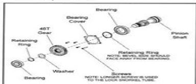
NOTE: If pinion shaft was disassembled, the bearing cover must be installed on the shaft before installing the 46T gear.
