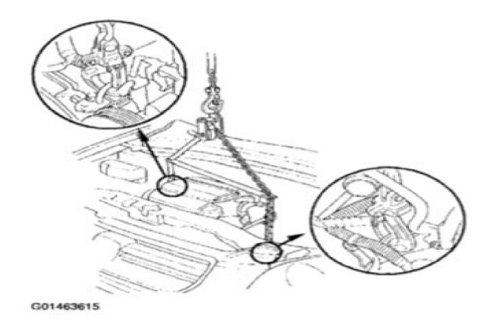
Fig. 28: Attaching The Chain Hoist To The Engine Courtesy of AMERICAN HONDA MOTOR CO., INC.
