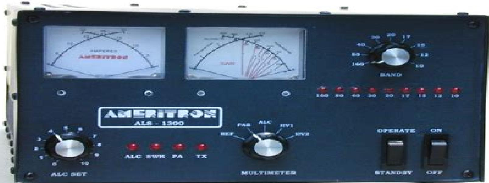
The Ameritron ALS-1300 is 160 through 15-meter amateur radio band 1200-watt output solid-state amplifier. It uses eight 50-volt conservatively rated linear RF MOSFETS. 50-volt linear FET's designed for transmitting service produce an exceptionally clean signal compared to other solid-state amplifiers. Fan speed is regulated by temperature sensors; assuring conservative cooling with minimum noise.
