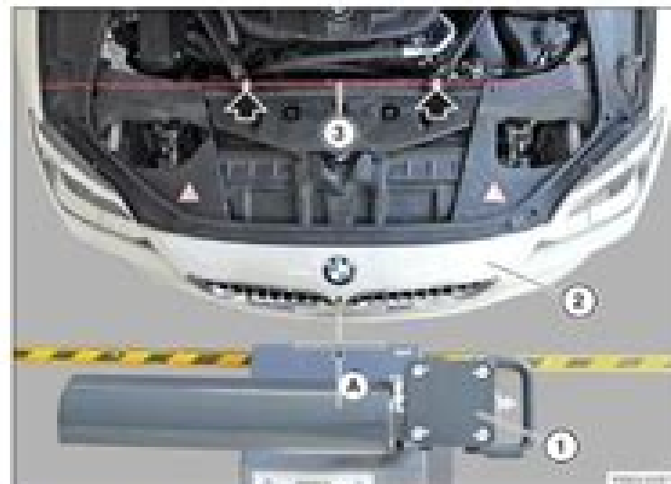
Fig. 16. Positioning Headlight Adjustment Device
