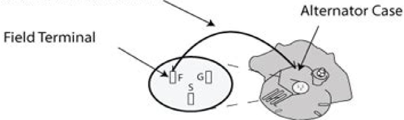
To field test a B circuit supply battery voltage to the field terminal.
