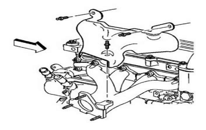
Fig. 1: Removing & Installing Exhaust Manifold Heat Shield Courtesy of GENERAL MOTORS CORP.
