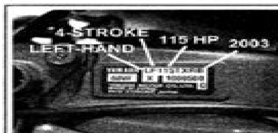
Fig. 3 The model ID tag provides critical information to identify and service the engine (4-stroke shown, but 2-stroke tags are mounted in the same way)
