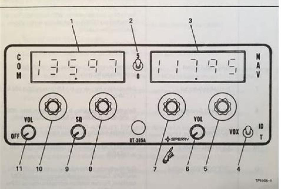
Figure 3-1. RT-385A Receiver-Transmitter, Controls and Indicators.
