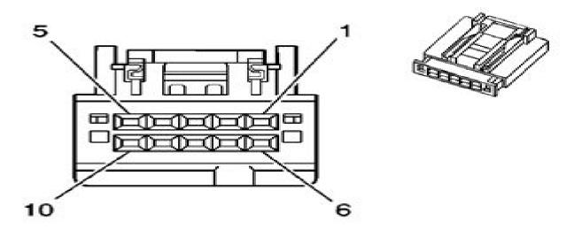
Fig. 4: Steering Wheel Control Switch Connector End View - Left
