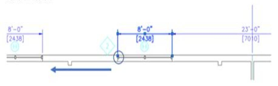
A CAD designer selects the bottom grip of a dimension as shown and moves the extension line to the left. How does this affect the selected dimension?
