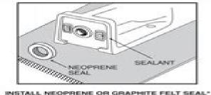
Install seal evenly around waste flange (horn). Apply a thin bead of sealant around base flange. "NOTE: Wax seal not recommended for this application.
