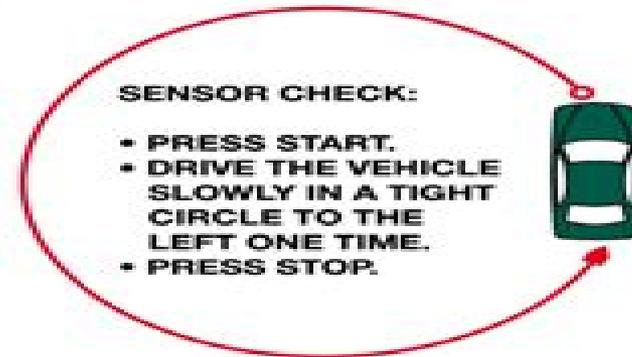
The test requires driving the vehicle in a tight circle at a speed of 6 MPH or less.
