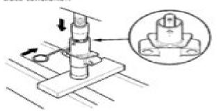
Use a hydraulic press to slowly compress the autotensioner. Insert a 2.0 mm (0.08 in.) pin through the housing and the rod.
