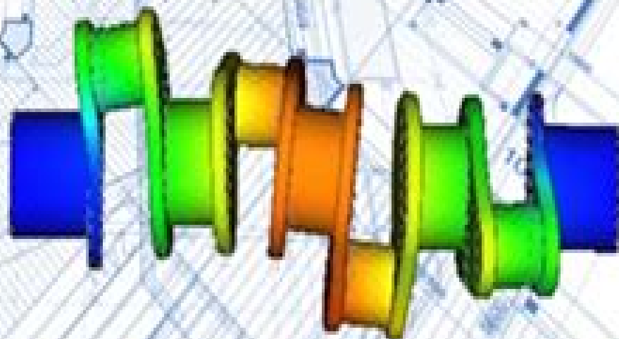
Mode Shape 2 - Frequency 151.7 Hz
