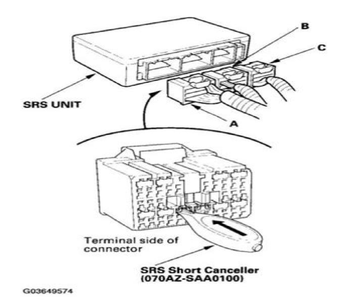
Fig. 20: Inserting SRS Short Canceller In Specified Cavities Courtesy of AMERICAN HONDA MOTOR CO., INC.
