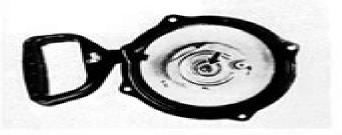
There is a drive plate spring and a drive pawl under the drive plate.
