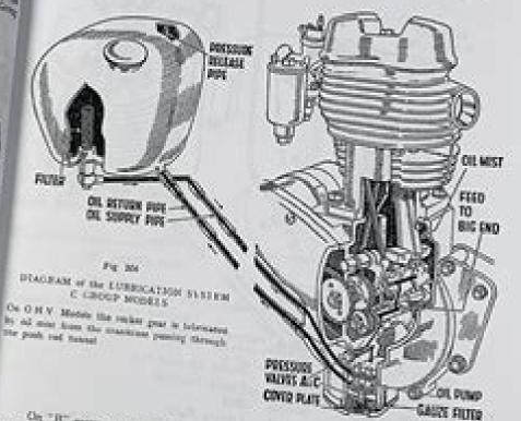
On "B" group machines od is fed through a union almosted in the pipe between the return pursup and the tank, to the cocker spindles, and after labricating the suckers and mentioned values, in enterneed to the crankdate through an entrust oil pape attached to the base of the solet valve spring bosong (see Fig M5). An internal solving connects.
