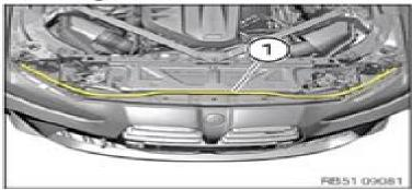
Detach the seal (1) upwards.
